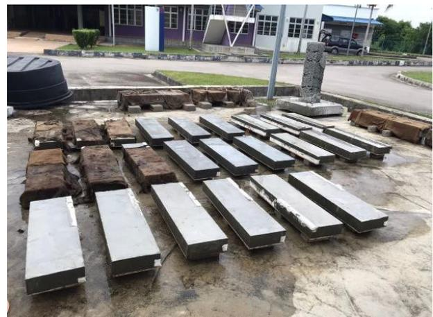
FIGURE 2. Curing of Wall Samples
