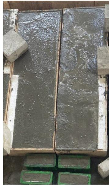
FIGURE 1. Casting of Wall Samples
