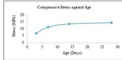
FIGURE 4. Compression Test Result
