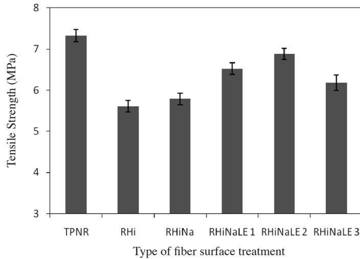
FIGURE 3. Tensile strength of TPNR and (NR/HDPE)/RH (90:10 v/v) composite, plotted as a function of RH surface treatment
