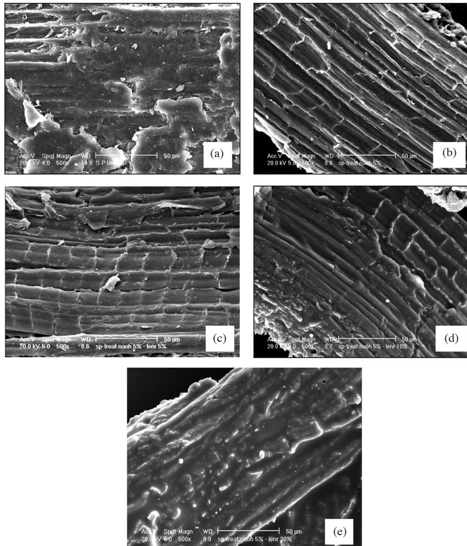
FIGURE 2. SEM micrographs of RH (a) RHi, (b) RHiNa, (c) RHiNaLE 1, (d) RHiNaLE 2 and (e) RHiNaLE 3
