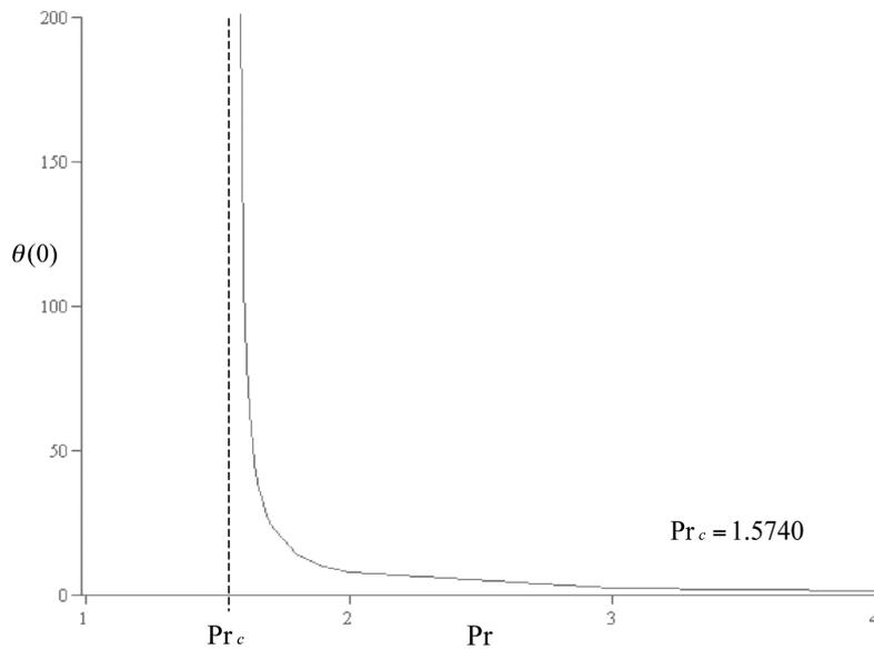
FIGURE 2. Variation of the surface temperature  $\theta(0)$  with Prandtl number  $Pr$  when  $\gamma = 1$  and  $\epsilon = 1$
