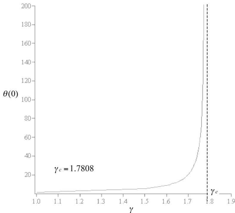
FIGURE 3. Variation of the surface temperature  $\theta(0)$  with conjugate parameter  $\gamma$  when  $\varepsilon = 1$  and  $Pr \approx 5$
