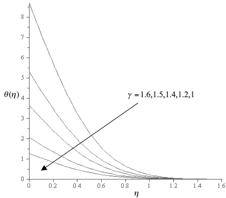
FIGURE 6. Temperature profiles  $\theta(\eta)$  for various values of  $\gamma$  when  $\varepsilon = 1$  and  $\text{Pr} = 5$
