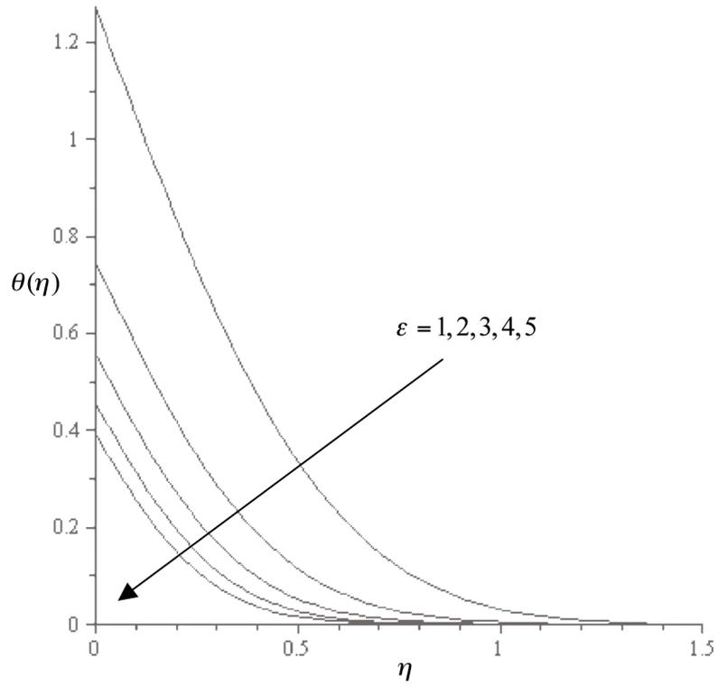
FIGURE 5. Temperature profiles  $\theta(\eta)$  for various values of  $\varepsilon$  when  $\gamma = 1$  and  $\text{Pr} = 5$
