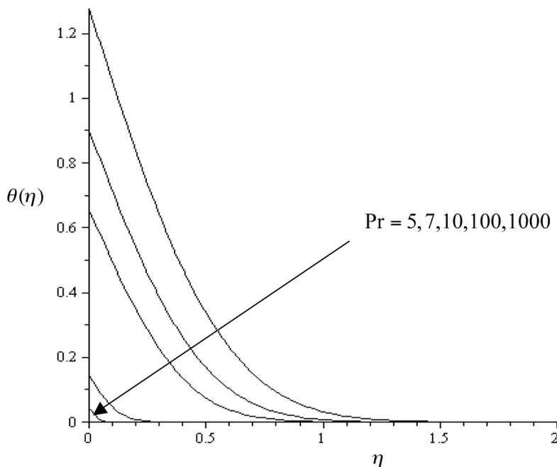
FIGURE 4. Temperature profiles  $\theta(\eta)$  for various values of  $Pr$  when  $\gamma = 1$  and  $\varepsilon = 1$
