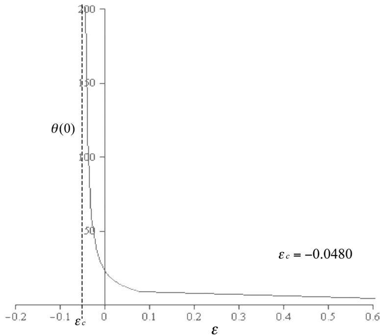
FIGURE 1. Variation of the surface temperature  $\theta(0)$  with  $\epsilon$  when  $\gamma = 1$  and  $Pr \approx 5$
