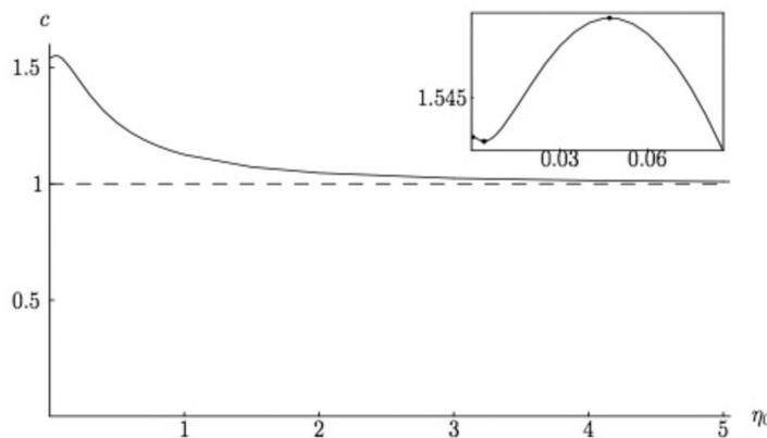
FIGURE 2. Plot of  $c$  as a function of  $\eta_0$ , together with the asymptotic value  $c = c_\infty = 1$  in the limit  $\eta_0 \rightarrow \infty$  (shown as a dashed line). The inset shows an enlargement of the behaviour near  $\eta_0 = 0$ ; the point  $c = c_0 \approx 1.5424$  at  $\eta_0 = 0$  is shown as a dot, as are the minimum  $c = c_{min} \approx 1.5421$  at  $\eta_0 \approx 0.0040$  and the maximum  $c = c_{max} \approx 1.5503$  at  $\eta_0 \approx 0.0470$
