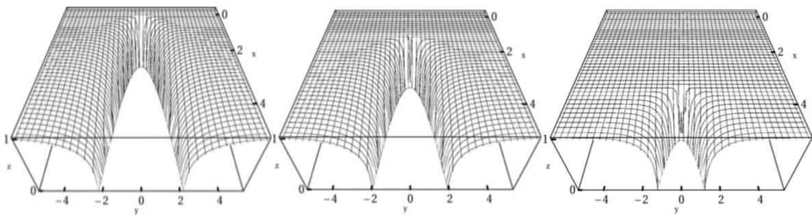
FIGURE 4. Three-dimensional plots of the free-surface profiles  $z = h$  in a sessile case with  $\eta_0 = 1$  at times  $t = 0, 3$  and  $5$
