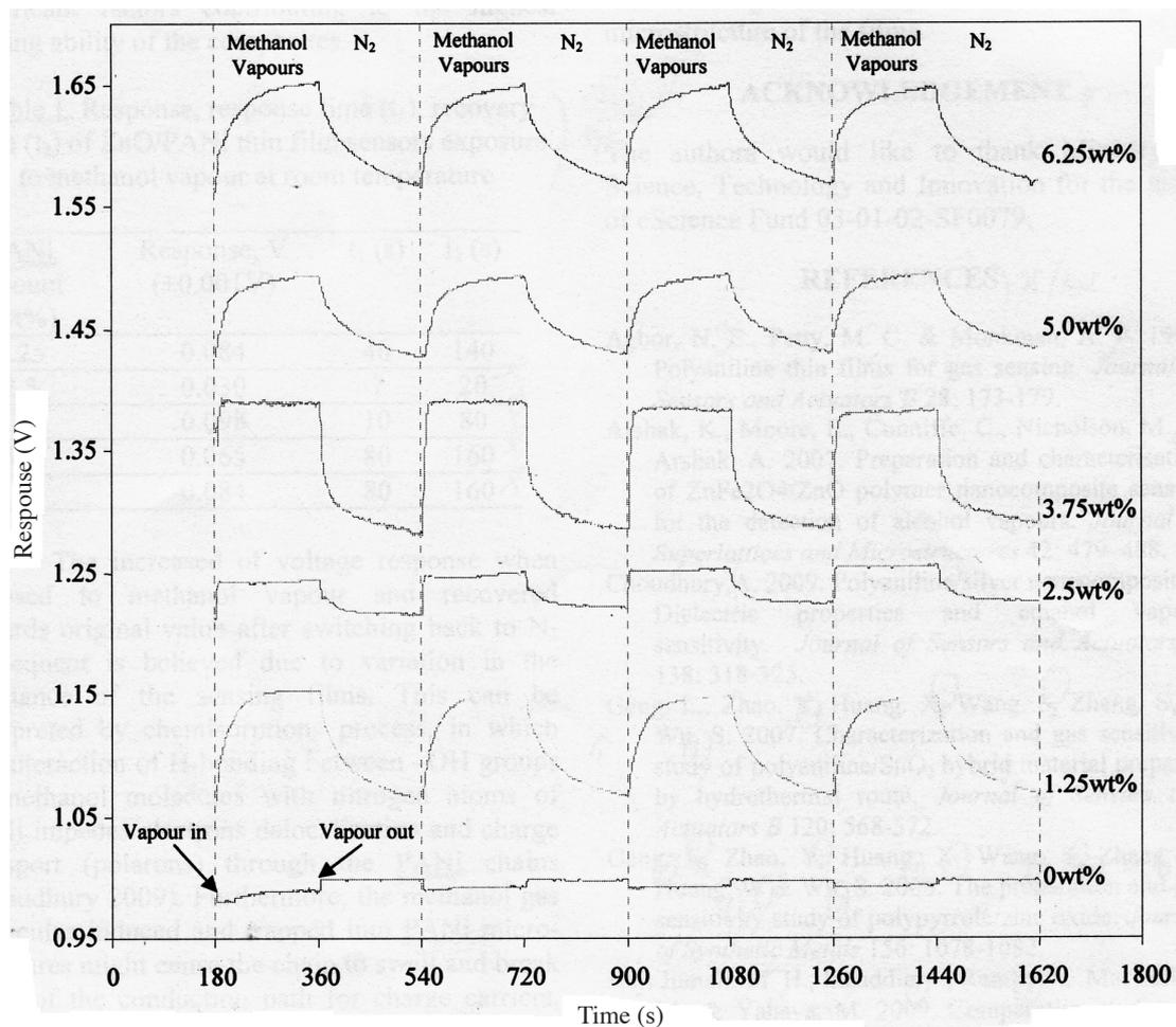
FIGURE 4. Sensor response of ZnO thin film with different weight percentage of PANI
