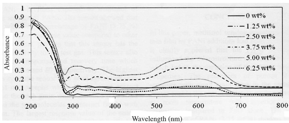
FIGURE 3. Variation of the UV-Visible absorption spectrum of ZnO as a function of weight percentage of PANI
