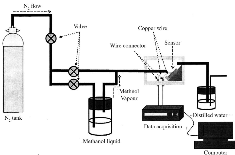
FIGURE 1. The sensing measurement setup
