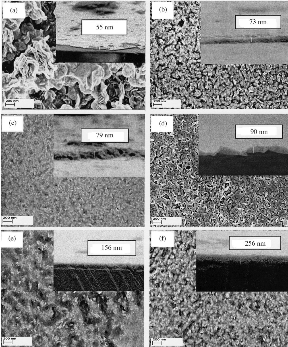
FIGURE 2. FESEM micrographs of ZnO thin film of (a) 0 wt% PANI (b) 1.25 wt% PANI (c) 2.50 wt% PANI (d) 3.75 wt% PANI (e) 5.00 wt% PANI (f) 6.25 wt% PANI and inset (upper right) shows the cross-sectional view of the films
