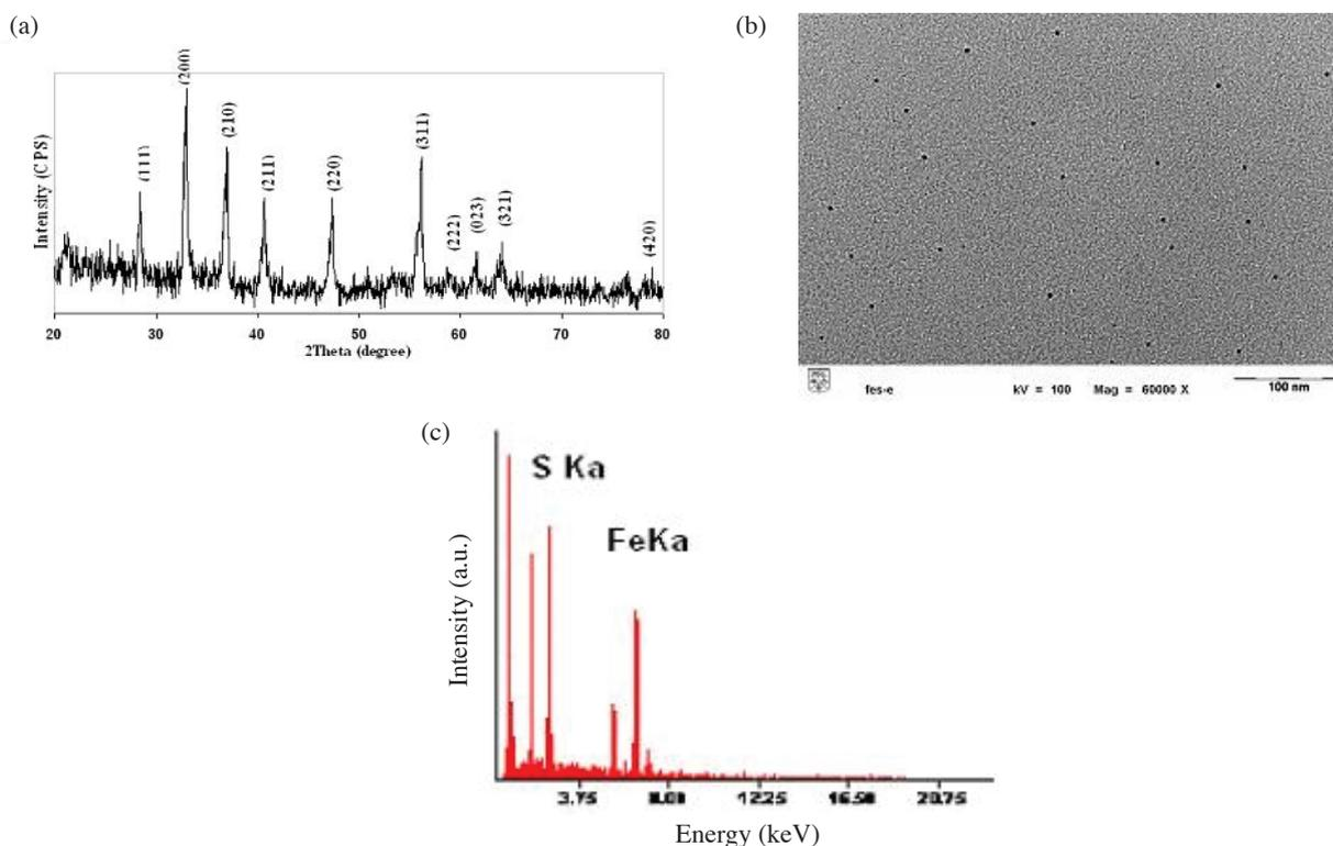
FIGURE 3. (a) XRD pattern of  $\text{FeS}_2$  nanoparticles with all the peaks indexed for the cubic pyrite  $\text{FeS}_2$  (JCPDS card 42-1340); (b) TEM image of  $\text{FeS}_2$  nanoparticles; and (c) EDX spectrum of  $\text{FeS}_2$  nanoparticles
