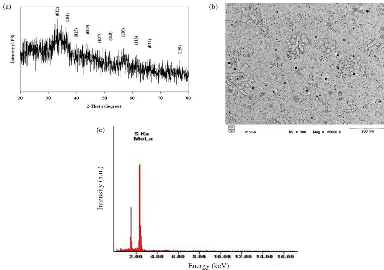
FIGURE 4. (a) XRD pattern of MoS<sub>2</sub> nanoparticles with all the peaks indexed for the rhombohedral molybdenite-3R (JCPDS card 17-0744) are shown for comparison, (b) TEM image of MoS<sub>2</sub> nanoparticles and (c) EDX spectrum of MoS<sub>2</sub> nanoparticles
