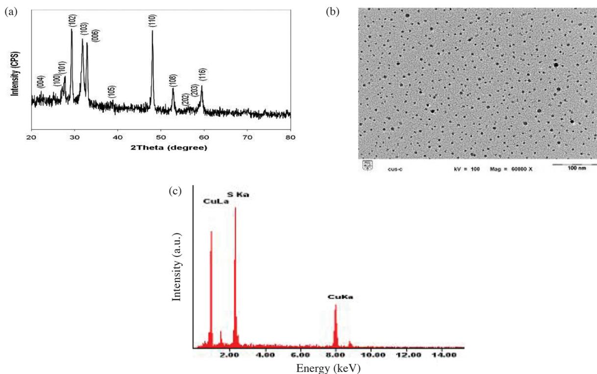
FIGURE 2. (a) XRD pattern of CuS nanoparticles with all the peaks indexed for the hexagonal covellite phase (JCPDS card 06-0464); (b) TEM image of CuS nanoparticles at 60000 $\times$  magnification; and (c) EDX spectrum of CuS nanoparticles
