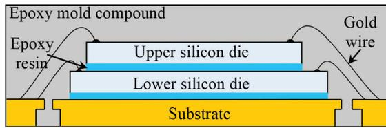
FIGURE 1. Cross section view of stacked die QFN
