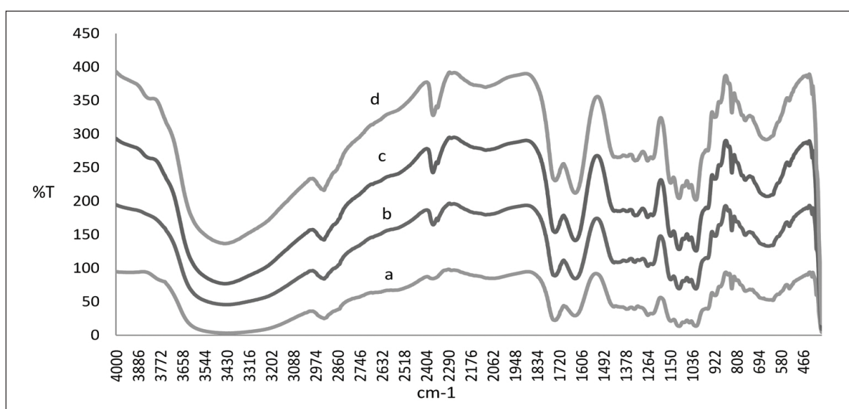
Fig. 2. FTIR spectra of (a) apple pectin from Sigma Inc., (b) dragon fruit pectin produced by ammonium oxalate extraction, (c) dragon fruit pectin produced by 0.03M HCl extraction, (d) dragon fruit pectin produced by deionised water extraction.
