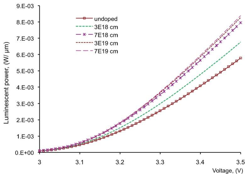
FIGURE 5. (Colour online) The luminescent power versus various doping concentrations in the selected quantum barriers for 5QWs
