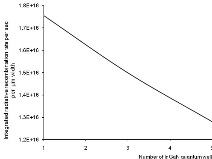
FIGURE 2. The dependence of radiative recombination in LED with different number of quantum well
