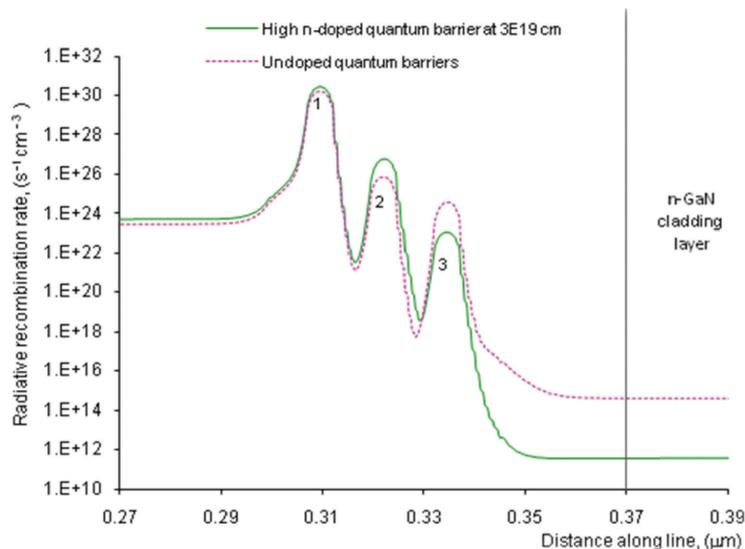
FIGURE 8. (Colour online) The distribution of radiative recombination rate for high n-doped quantum barrier and undoped quantum barrier for the 3QWs LEDs. The wells are numbered in the figure
