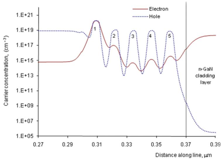
FIGURE 4. (Colour online) The distribution of electron and hole concentration for 5QWs LEDs at applied voltage of 3.5 V. The wells are numbered in the figure
