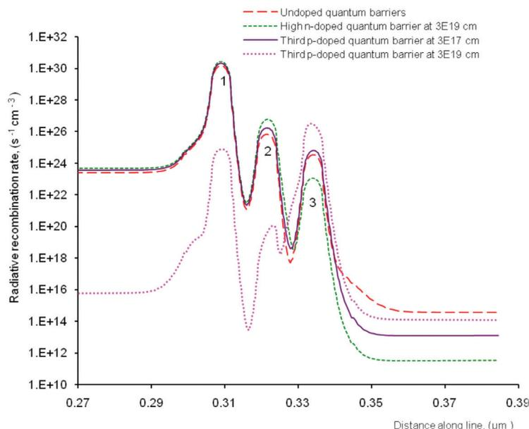
FIGURE 9. (Colour online) The distribution of radiative recombination rate for LEDs structure for various doping in the selected quantum wells for the 3QWs LEDs. The wells are numbered in the figure
