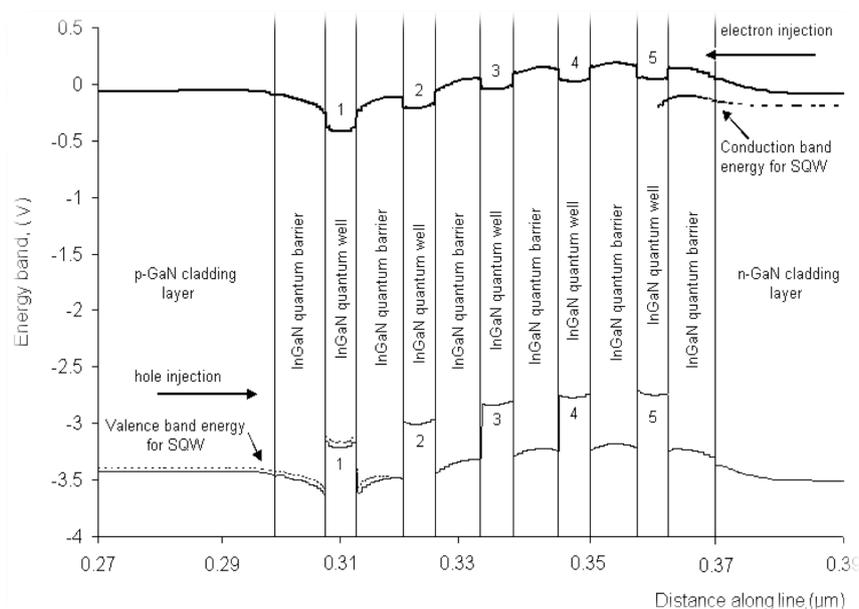
FIGURE 3. The conduction and valence band for 5QWs and SQW at applied voltage of 3.5 V. Quantum wells are numbered as 1, 2, 3, 4 and 5
