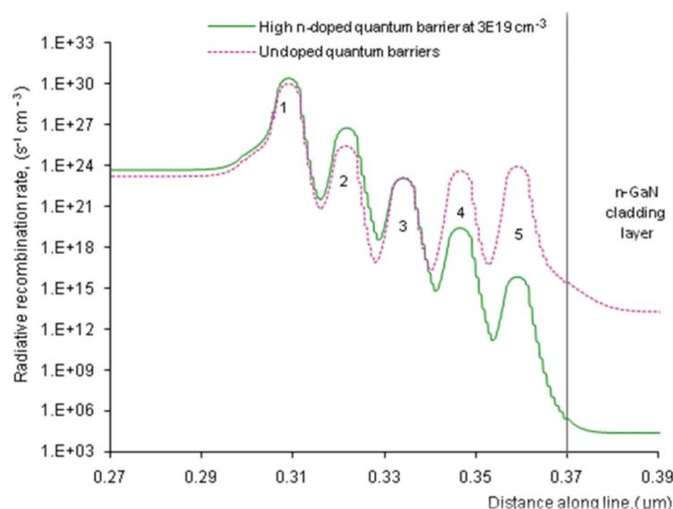
FIGURE 7. (Colour online) The distribution of radiative recombination rate for high n-doped quantum barrier and undoped quantum barrier for 5QWs LEDs. The wells are numbered in the figure
