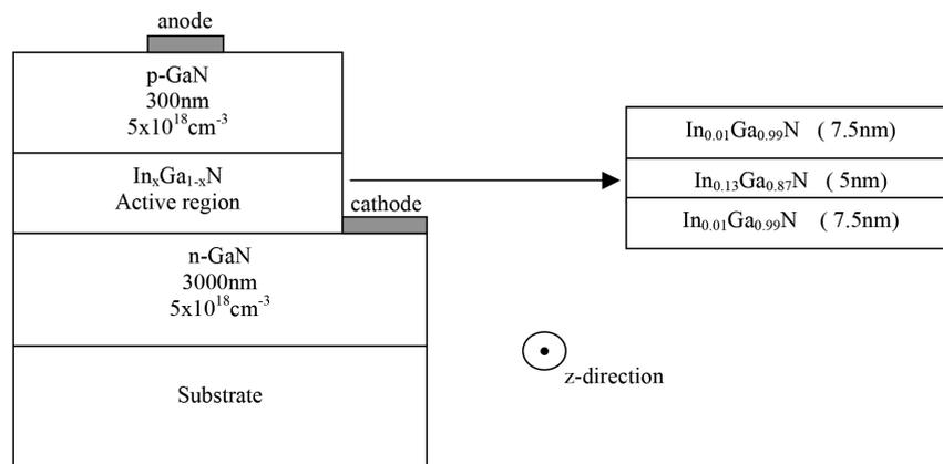
FIGURE 1. LEDs structures for single (SQW) and multi quantum wells (MQWs) in the active region
