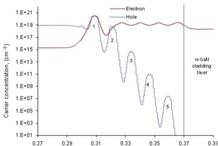
FIGURE 6. (Colour online) The distribution of carrier's concentration for LED with 5QWs with an increased doping of  $3.0 \times 10^{19} \text{ cm}^{-3}$ . The wells are numbered in the figure
