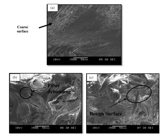
FIGURE 3. Tensile fracture surface of LDPE/SSP with a) 0% SG loading, b) 5% SG loading and c) 15% SG loading
