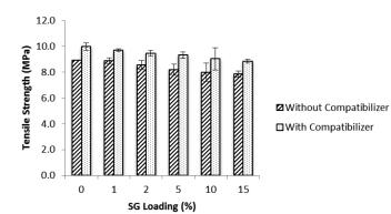
FIGURE 1. Comparison of tensile strength for uncompatibilized and ENR 50 compatibilized SG filled LDPE/SSP composites
