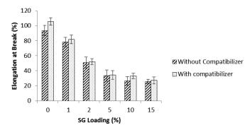
FIGURE 2. Comparison of  $E_b$  for uncompatibilized and ENR 50 compatibilized SG filled LDPE/SSP composites
