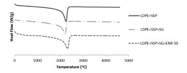
FIGURE7. DSC cooling thermogram of SG filled LDPE/SSP
