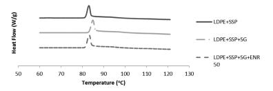
FIGURE 6. DSC melting thermogram of SG filled LDPE/SSP
