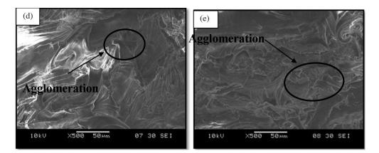
FIGURE 4. Tensile fracture surface of LDPE/SSP with d) 5% SG and 0.5% ENR 50 and e) 15% SG and 0.5% ENR 50
